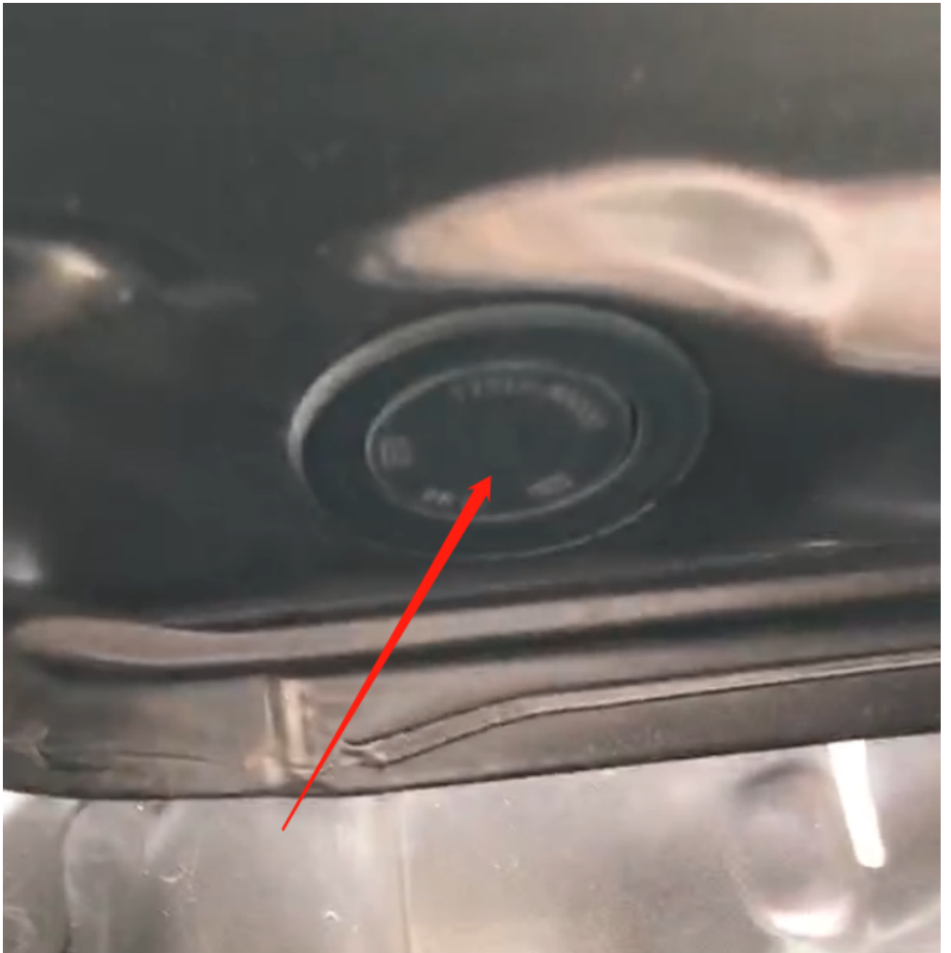
撑杆线从上图原车孔进入The strut line enters from the original car hole in the above picture
