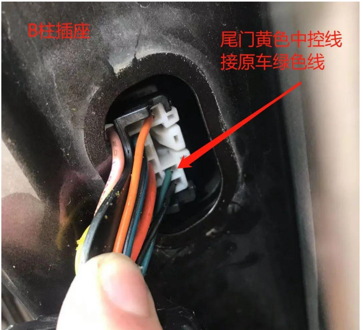
左侧B柱波纹管处：尾门黄色中控线接原车绿色线 At the bellows of the left B-pillar: the yellow central control line of the tailgate is connected to the green line of the original car
