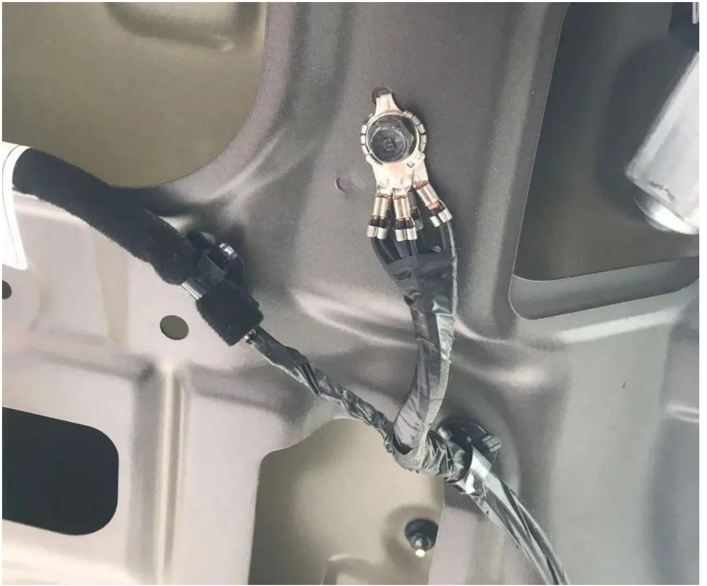
车尾尾门内部接地Internal grounding of rear tailgate
